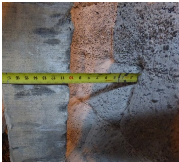
Figure 3 – Advance lining's wear of slag line at strength of 50 melts within the area of a blowing plug
